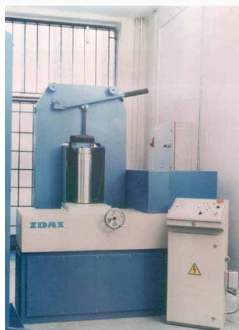
Figure 4: A laboratory isostatic press, CYX 6/106 (Ždas a.s., ČR)
