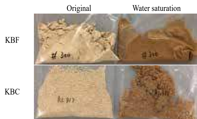
Figure 1. Kieselguhr before and after water saturation.
